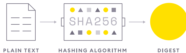
Fig. 3: Cryptographic Digests. A cryptographic digest process takes plain text and generates a string unique to that input text, which acts as a digital fingerprint.
